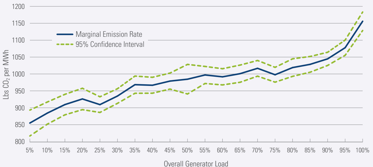
FIGURE 3: Average CO 2 Marginal Emission Rates as a Function of Overall Generator Load
